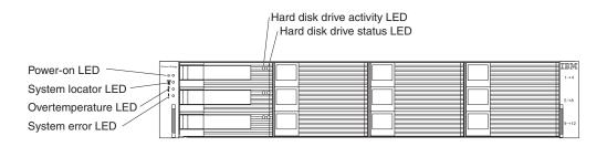
Figure 35. Front LEDs and controls
